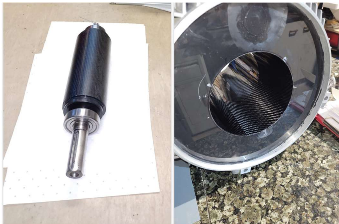
Fig. 1. Custom ferrofluid-gap test generator rotor (left) and stator (right).
